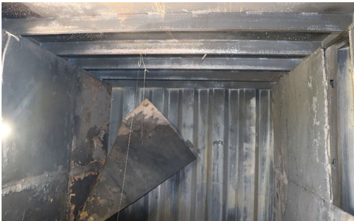
FIGURE 7 Interior of steel BRM after external jet fire.
