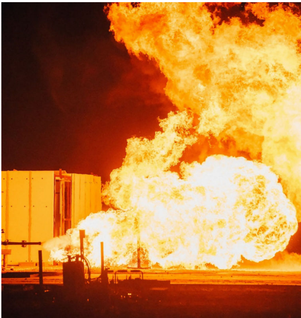
FIGURE 6 Jet fire test from BakerRisk's Wilfred E. Baker test facility.
