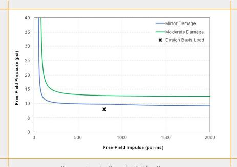
Pressure-Impulse Curve for Building Damage
